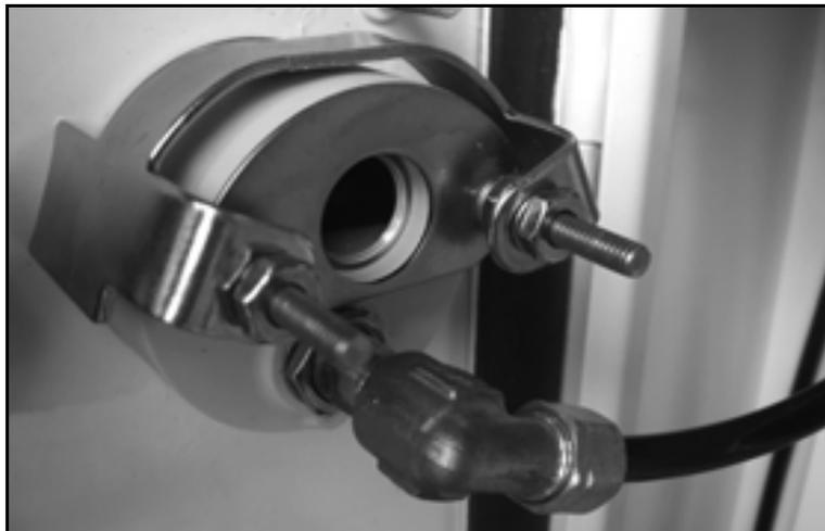
*Figure 7-10. Remove the hose from the vacuum gauge, then remove the nuts holding it to the bracket.*
