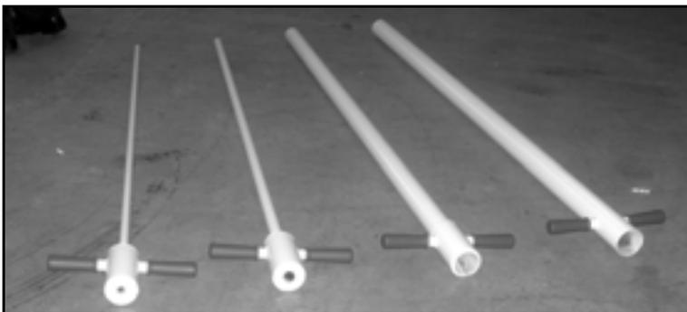
*Figure 3-10. Various sized vacuum wands are available. All wands are fitted to the 3" vacuum hose.*
