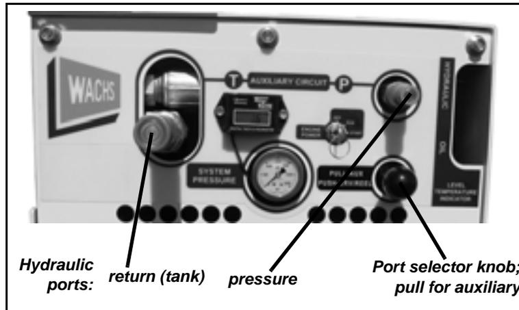
*Figure 5-48. Connect hoses to the hydraulic ports and pull out the port selector knob.*
