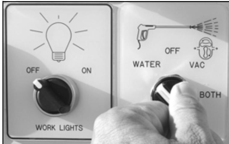
*Figure 5-36. Turn the pressure washer switch to the WATER position.*
