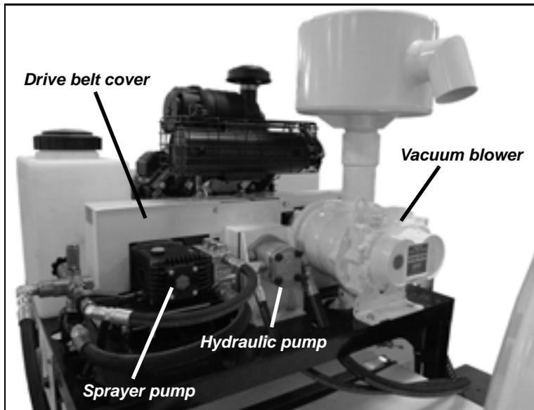
Figure 3-4. The vacuum blower, hydraulic pump, and sprayer pump as seen from behind the engine.
