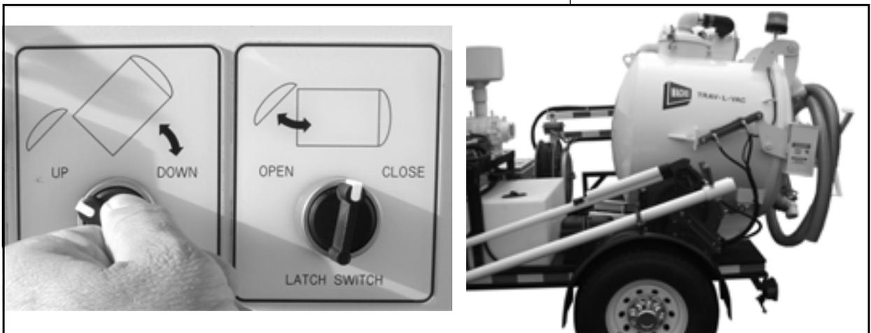
*Figure 5-22. Turn the Dump Switch to the UP position and hold it **just until the tank has cleared the deck and begins to tip** (approximately 10° - 20°).*
