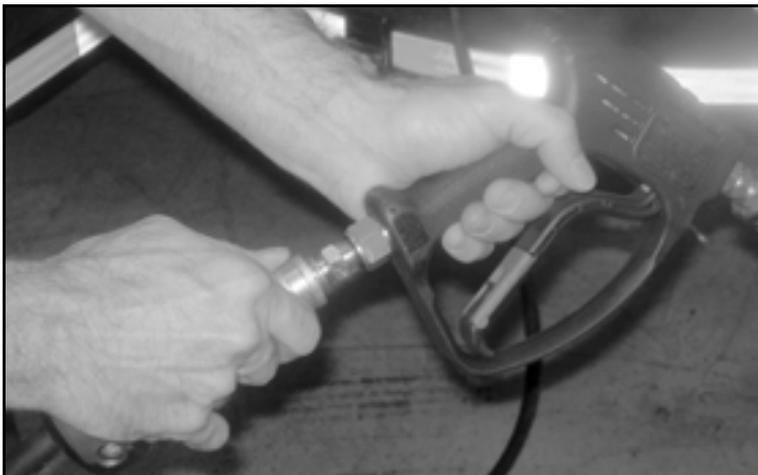
*Figure 5-35. Attach the spray wand to the sprayer hose.*
