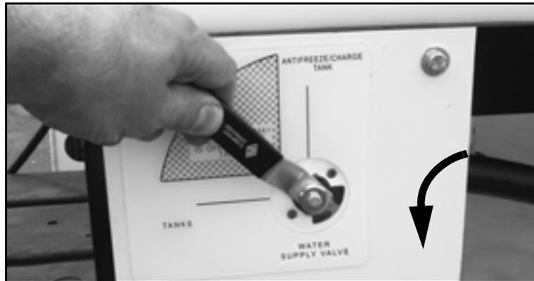
*Figure 4-1. Move the Water Supply Valve to the TANKS position.*
