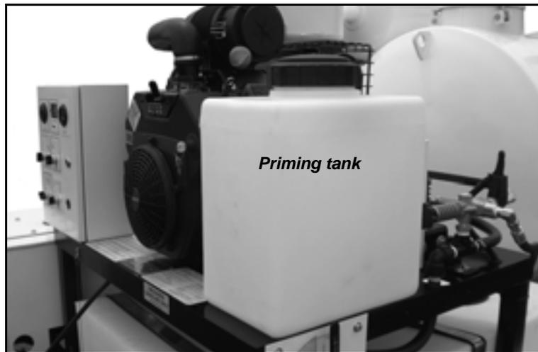
*Figure 5-33. Fill the priming tank with either anti-freeze (when using the system in freezing weather) or water treated with a purifying agent (when using the system in non-freezing weather.)*
