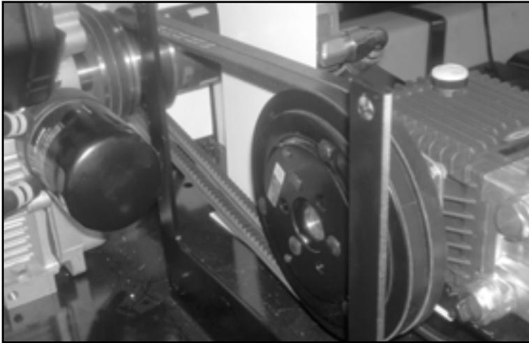
*Figure 7-23. Inspect the sprayer pump belts for damage and correct tension.*
