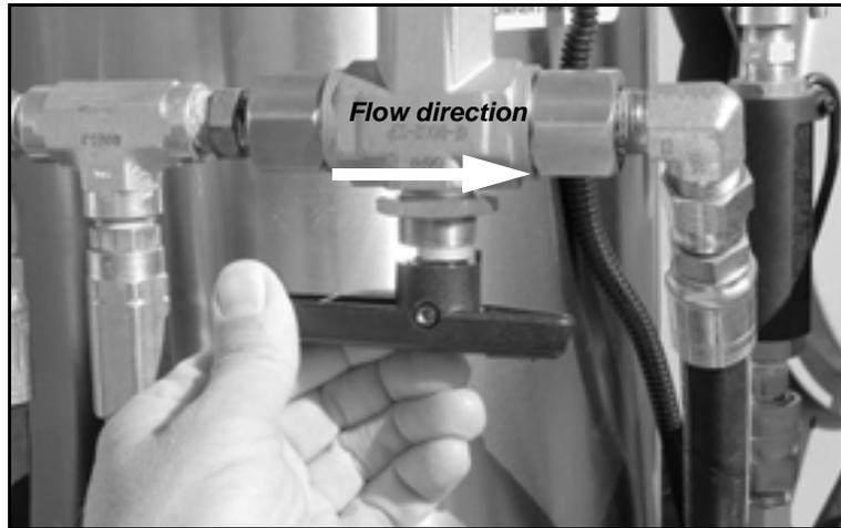
*Figure 4-9. Turn the heater valve to direct the flow direction to the right. The flow is toward the shorter end of the handle.*
