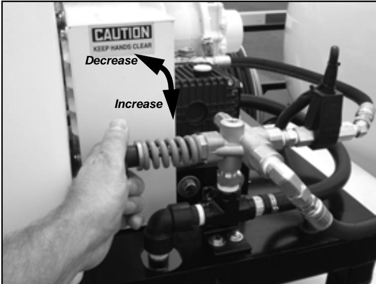
*Figure 5-38. Turn the unloader knob clockwise to increase the water pressure, or counter-clockwise to decrease water pressure.*
