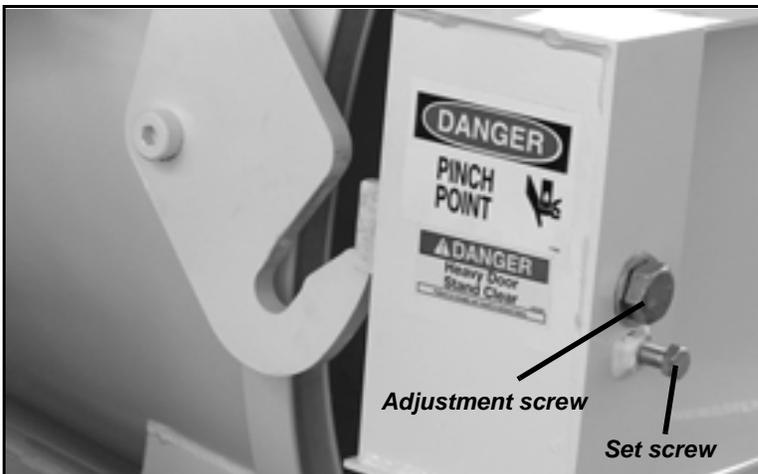
*Figure 7-26. The front of the latch cover has screws for adjusting the latch.*
