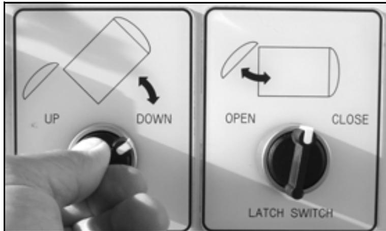
*Figure 5-27. After the tank is dumped, turn the Dump Switch to the DOWN position until the tank has moved back to its operating position.*
