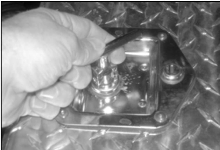
*Figure 5-3. Lift the handle and turn it to open the job box.*
