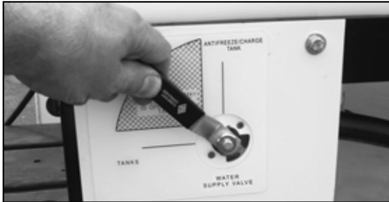
*Figure 4-13. Move the Water Supply Valve to the TANKS position.*
