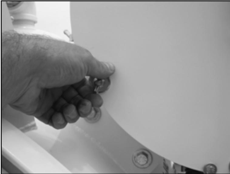
*Figure 6-2. Loosen the wing nuts securing the filter canister cover.*
