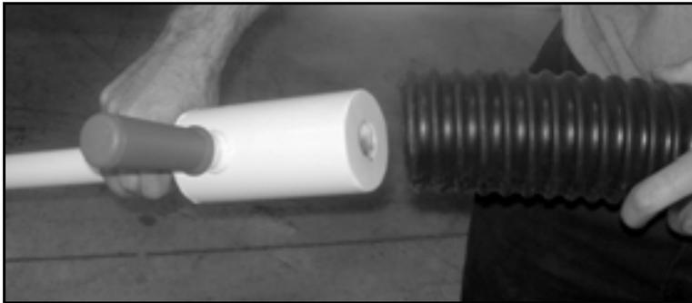
*Figure 5-11. Insert the wand fitting into the end of the vacuum hose.*
