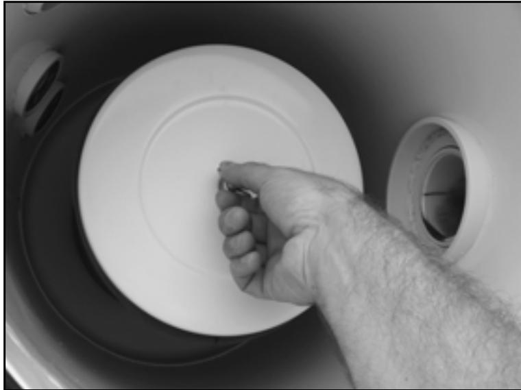
*Figure 6-4. Remove the knob holding the filter in place. Be careful not to lose the washer behind the knob.*
