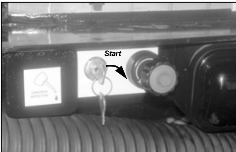
Figure 5-7. Turn the engine key to *START*. Release it to *RUN* when the engine starts.
