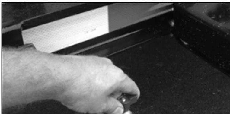
*Figure 4-5. Open the drain valve on the back of the trailer to drain the water tank.*
