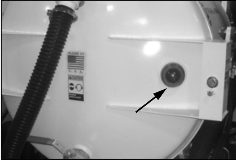
Figure 5-15. Monitor the fill level of the tank using the sight glass.
