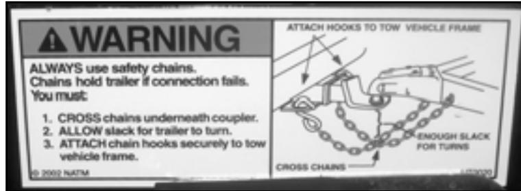
Figure 2-11. The safety chain warning label is on the tongue of the trailer. (Part no. 77-160-20.)
