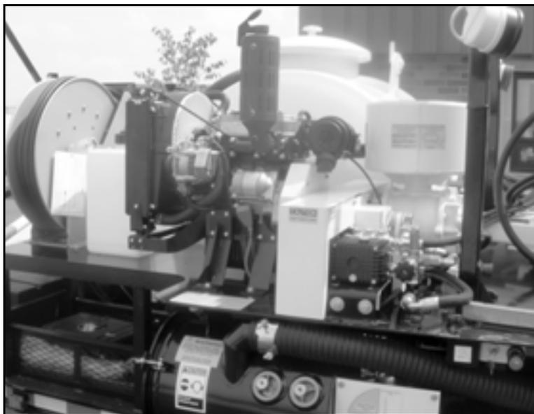
*Figure 3-6. The diesel engine is shown. The engine keyswitch and throttle are located remotely.*
