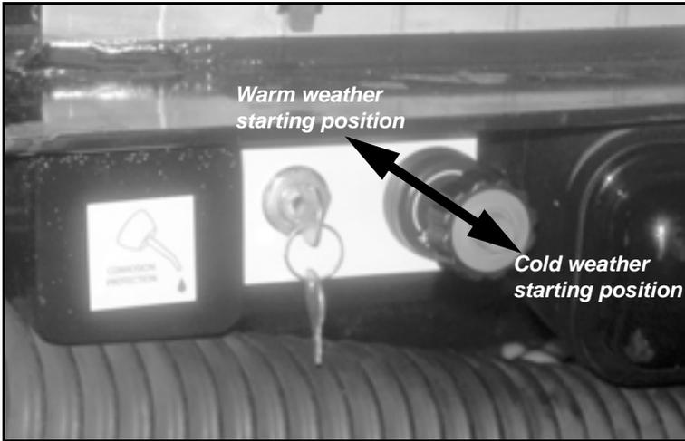
Figure 5-6. Push the throttle knob (at right) in to start the engine in warm weather; pull the knob out to start the engine in cold weather.
