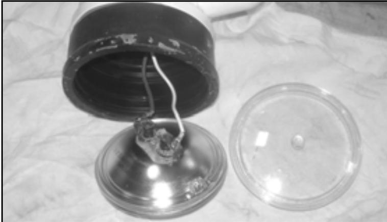
*Figure 7-35. Pull the cover and bulb out of the rubber seal around the lamp housing.*
