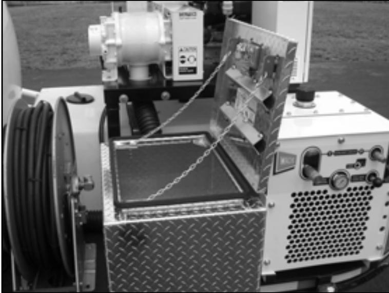
*Figure 3-15. The optional locking job box is mounted on the front of the trailer.*
