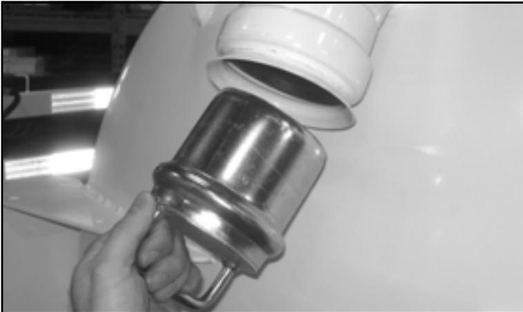
*Figure 5-9. Remove the plug from the inlet port.*
