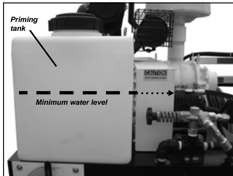
*Figure 5-40. Fill the priming tank so that the water level is above the pump.*
