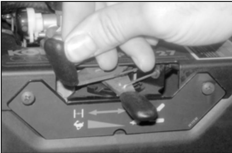
*Figure 5-4. To start the engine, set the choke lever (top) all the way to the left, and the throttle lever (bottom) in the middle.*
