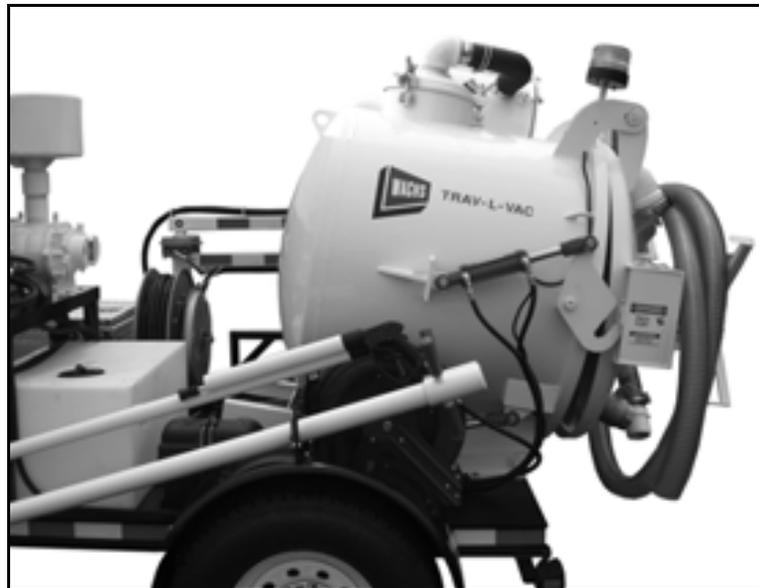
*Figure 5-24. The tank door will swing open when the latches are released.*
