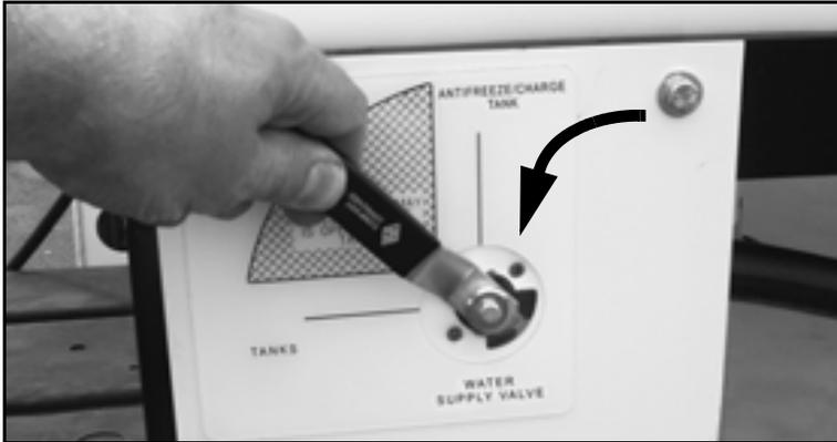
*Figure 5-45. Move the Water Supply Valve lever to the TANKS position to prime the main tank.*
