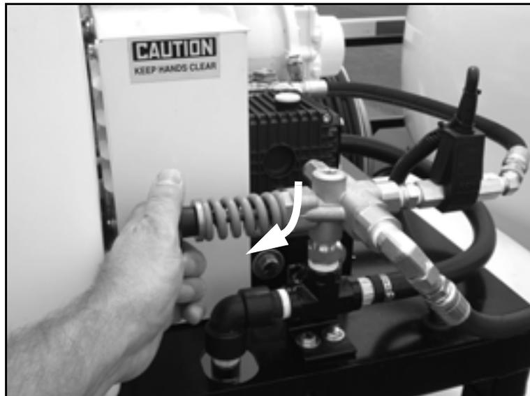
*Figure 5-44. Turn the unloader knob clockwise to increase the water flow.*
