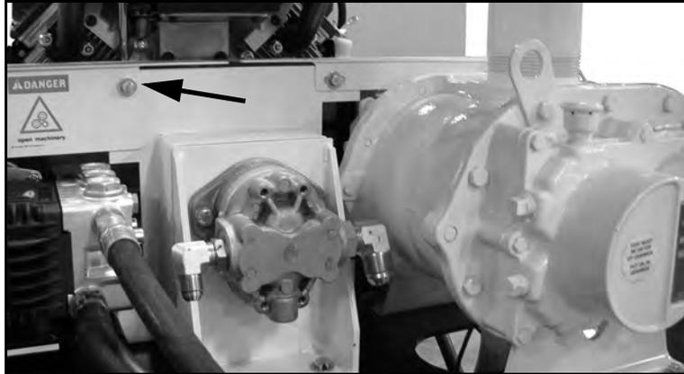
*Figure 7-21. Remove the screw on the back of the sprayer pump belt cover.*
