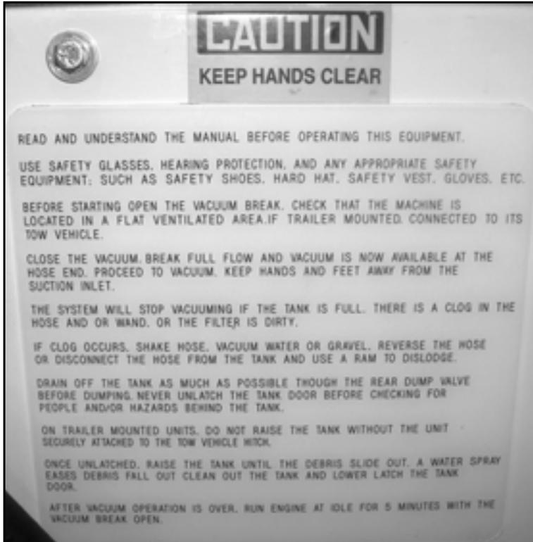
*Figure 2-3. The safety and instruction label is on the engine deck plate. It lists operating and general safety guidelines. (Part no. 77-094-00.)*
