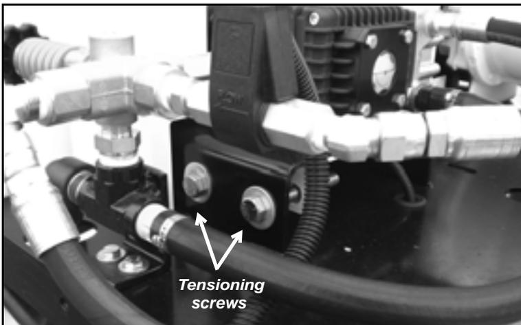
*Figure 7-24. Turn the tensioning screws counter-clockwise to loosen the tension on the belts.*
