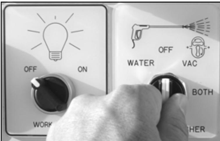
Figure 5-16. Turn the Vacuum/Pressure Washer switch OFF to turn off the vacuum.
