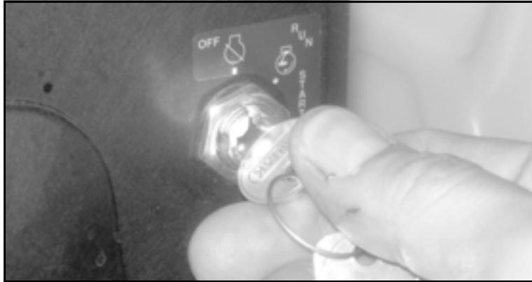
*Figure 5-5. Turn the engine key to START. Release it to RUN when the engine starts.*
