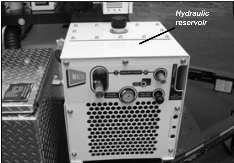
Figure 3-12. The hydraulic system reservoir.
