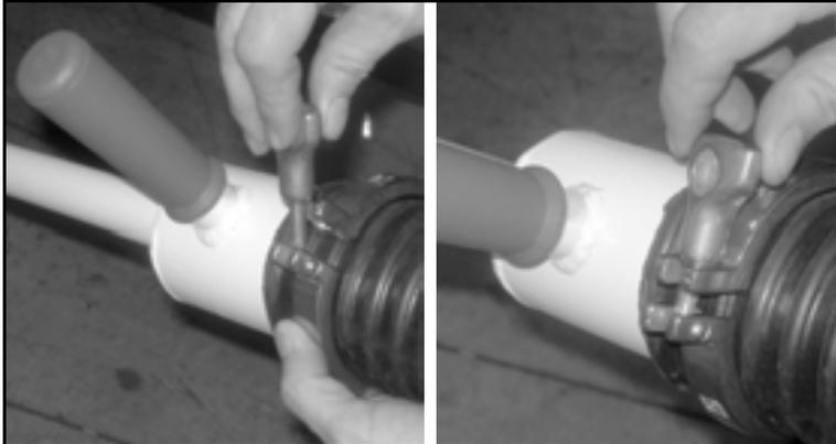
*Figure 5-12. Attach the hose to the wand using the hose clamp.*
