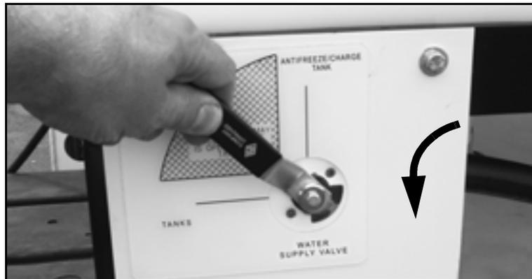
*Figure 4-6. Move the Water Supply Valve to the TANKS position.*
