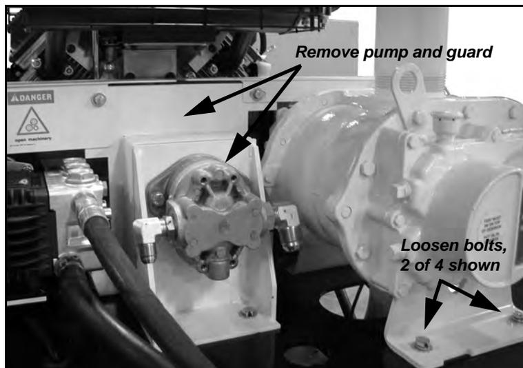
*Figure 7-20. Loosen the four bolts holding the blower to the engine platform (two are shown). Remove the hydraulic pump and guard.*
