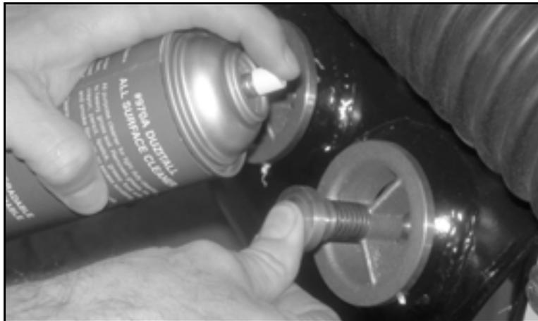
*Figure 6-15. Spray lubricant on the pressure relief valves.*
