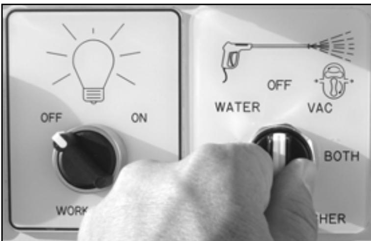
*Figure 5-39. Turn the Vacuum/Pressure Washer switch OFF when finished spraying.*
