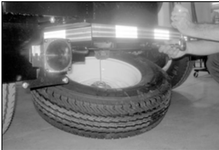
*Figure 5-1. Turn the cable release nut to lower the spare tire to remove it.*
