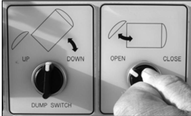
*Figure 5-23. Turn the Latch Switch to the OPEN position and hold it until the door swings open.*
