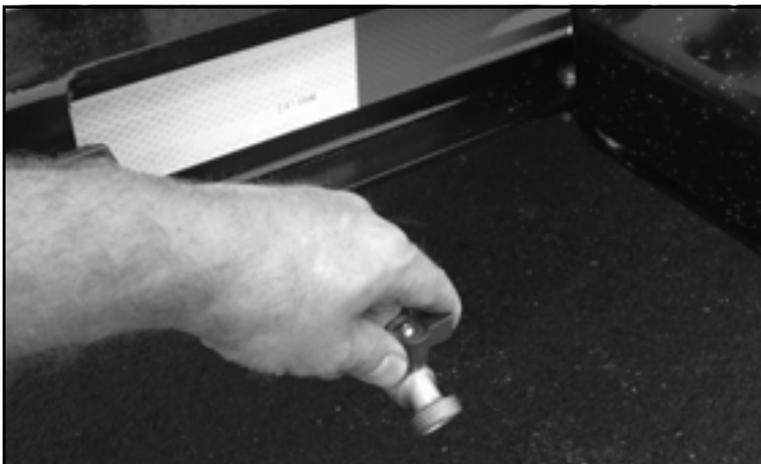
*Figure 4-12. Open the drain valve on the back of the trailer to drain the water tank.*
