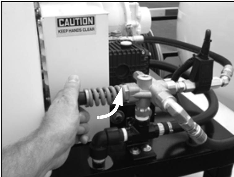
Figure 5-42. Turn the unloader knob counter-clockwise until the spring tension is released.
