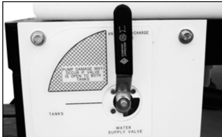
*Figure 4-3. Move the Water Supply Valve to the ANTI-FREEZE/CHARGE TANK position.*
