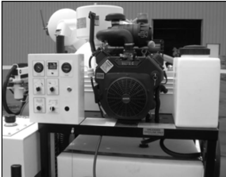
*Figure 3-5. The gasoline engine, shown in the center, powers all of the equipment provided with the VMT-2.*
