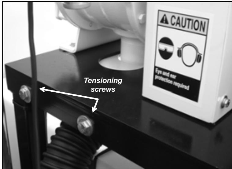
*Figure 7-19. The blower belt tensioning screws are located on the right side of the trailer just beneath the vacuum blower.*
