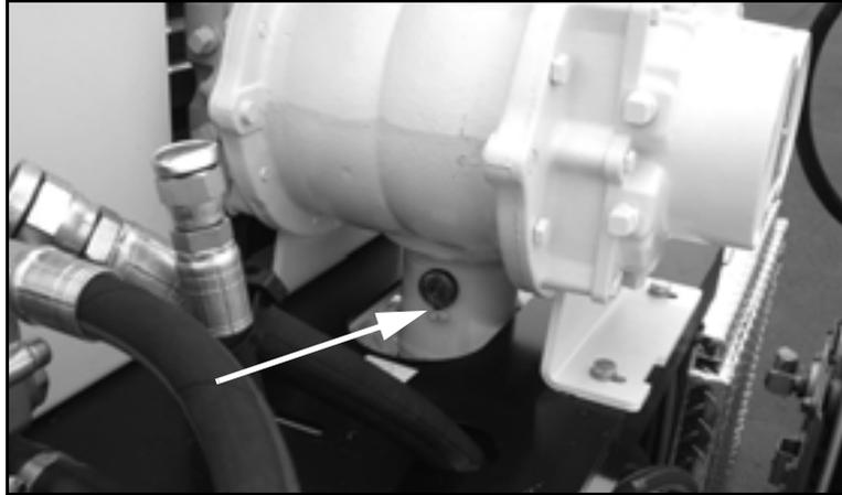
*Figure 6-6. Access the blower lubrication port from the rear of the engine platform.*
