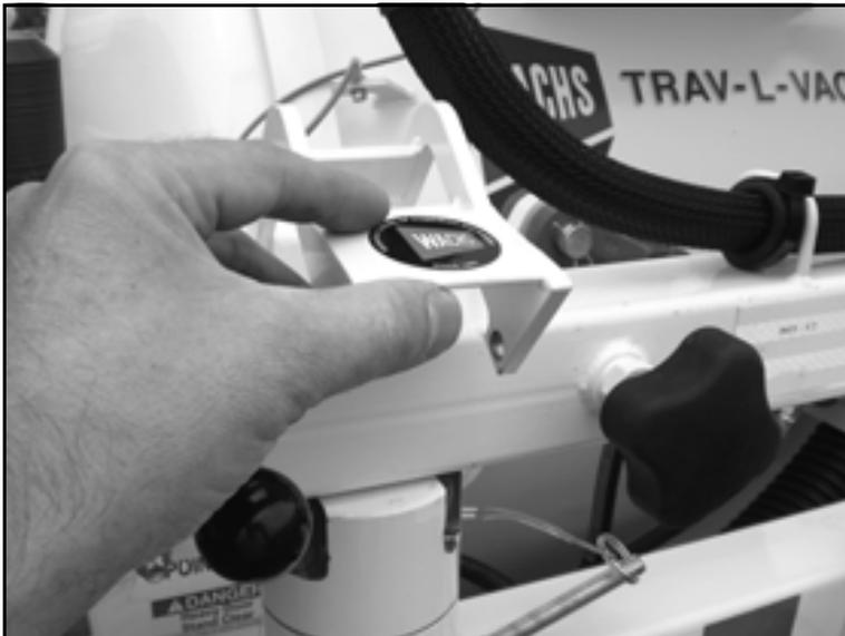
*Figure 5-62. Lift the latch up and over the arm.*
