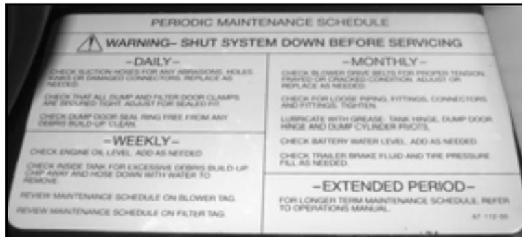
Figure 2-12. This label is on the trailer deck next to the engine. Shut the system down before performing service. (Part no. 67-112-00.)
