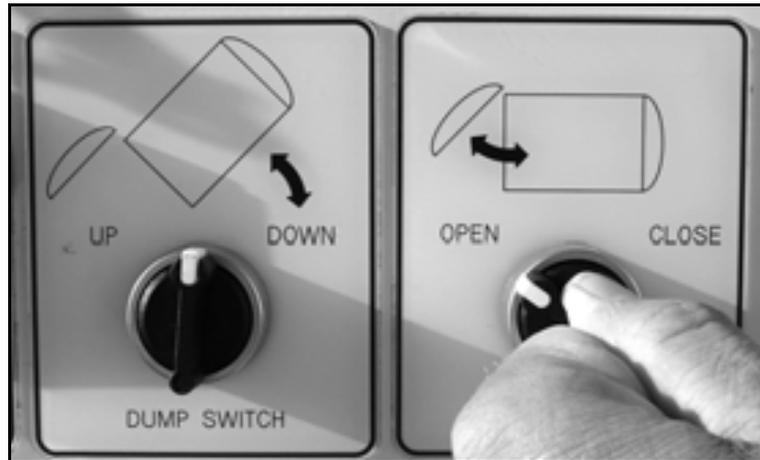
*Figure 7-27. Turn the Latch Switch to the OPEN position and hold it until the latch fully opens.*
