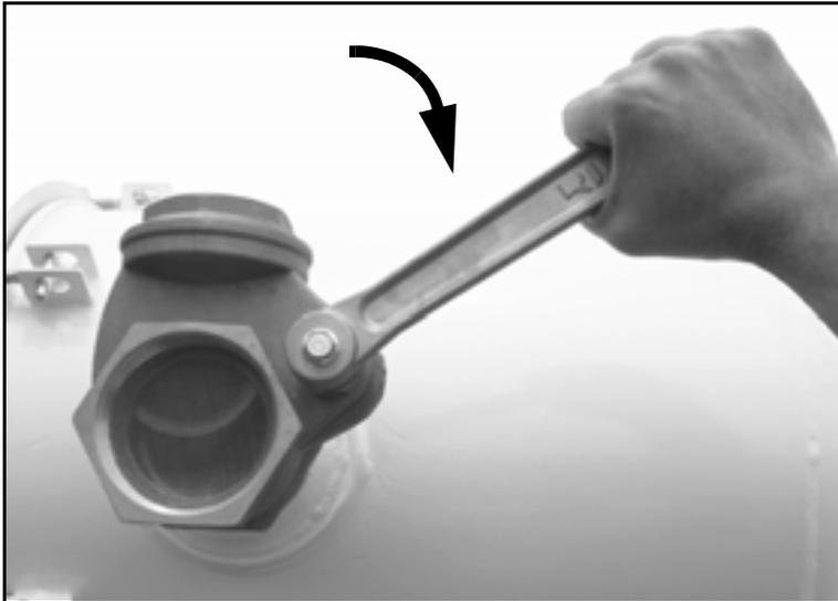
*Figure 5-29. Turn the Vacuum Break lever to the CLOSED position.*
