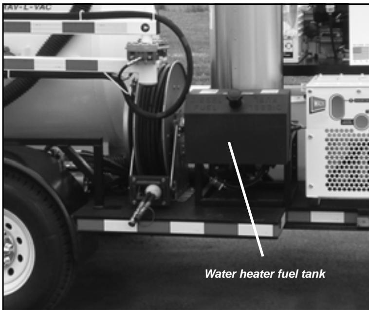
*Figure 5-50. The water heater fuel tank is mounted in front of the heater.*
