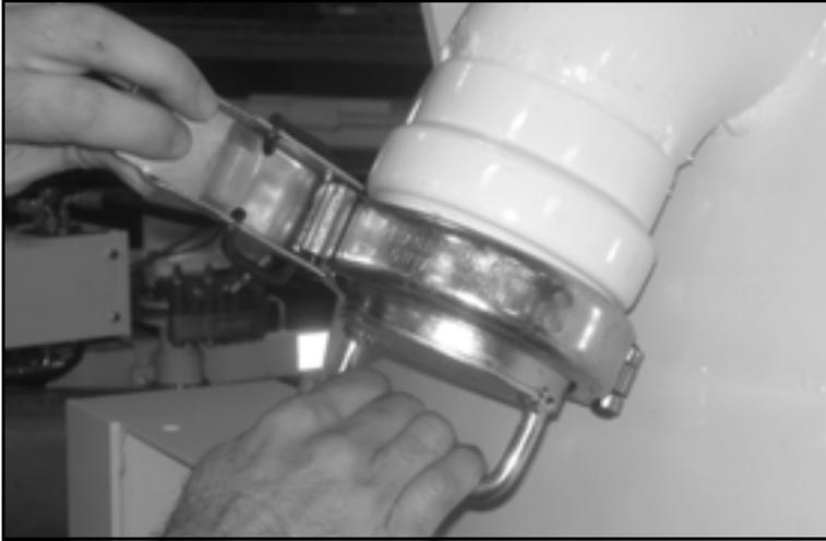
*Figure 5-8. Pull the latch on the locking collar to release it and take it off the inlet port.*
