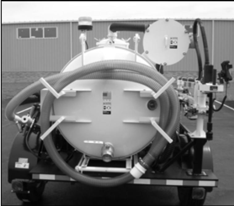
*Figure 3-9. The vacuum hose is rolled up and stored on the rear of the trailer.*
