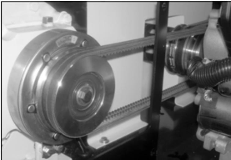
*Figure 7-18. Inspect the blower belts for damage and correct tension.*
