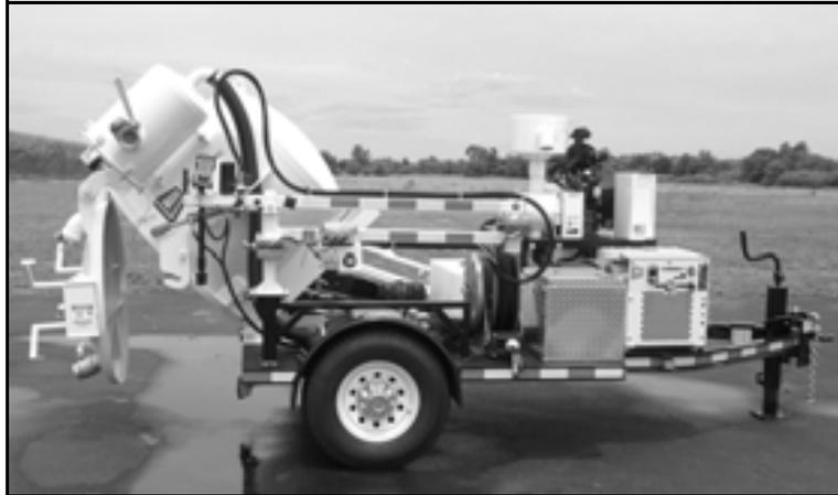
*Figure 3-7. The tank dumping mechanism moves the tank to the rear of the trailer, opens the door latch, and tips the tank for dumping.*
