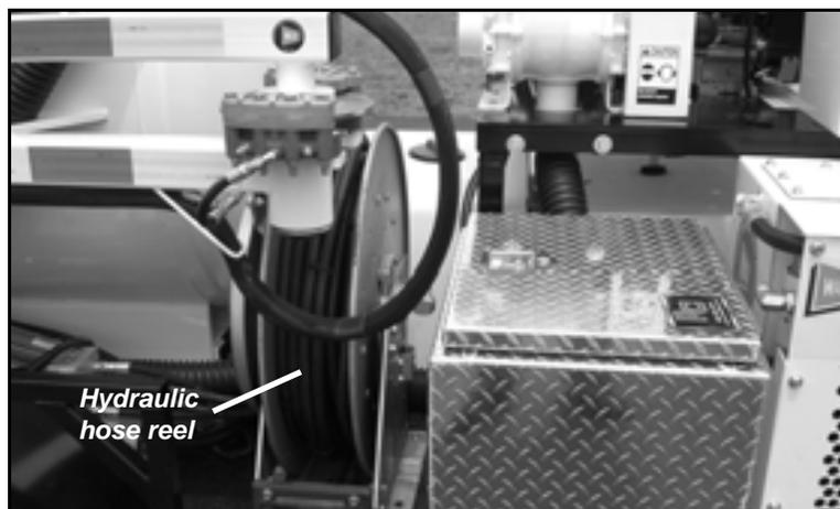
*Figure 3-14. The auxiliary hydraulic hose reel is mounted on the front of the trailer.*
