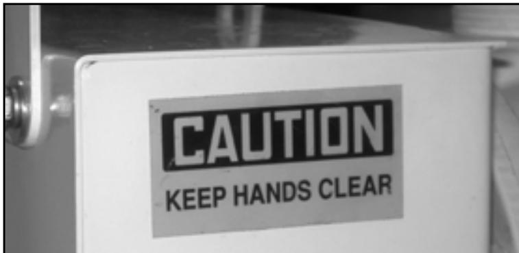
*Figure 2-4. This caution label is on the left-hand side of the pressure washer belt guard. Keep hands away from the belt drive area while any equipment is operating or the gas engine is running. (Part no. 77-160-11.)*
