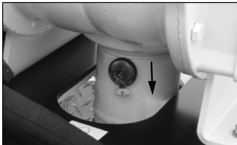
*Figure 6-11. Flip the tab down to lock the plug.*
