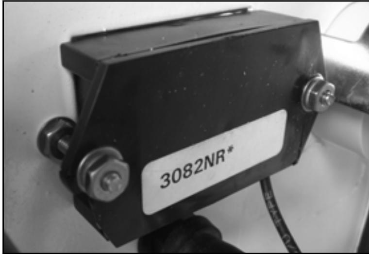
*Figure 7-9. Remove the nuts to take off the tach/hour meter.*
