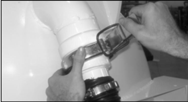
*Figure 5-10. Insert the hose fitting into the inlet port and attach it with the locking collar.*
