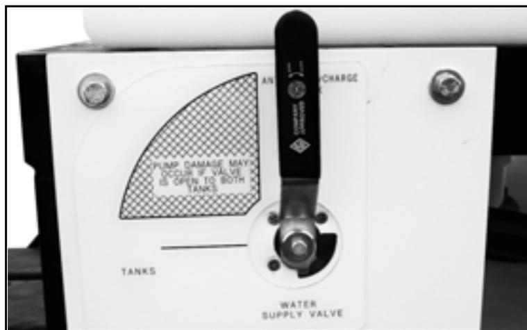
*Figure 4-10. Move the Water Supply Valve to the ANTIFREEZE/CHARGE TANK position.*
