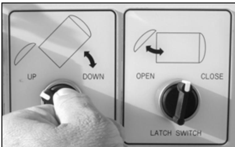
*Figure 5-25. After opening the tank door, turn the Dump Switch to the UP position to completely tip the tank.*
