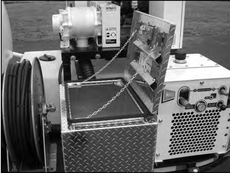
*Figure 5-2. The optional job box is mounted at the front of the trailer.*
