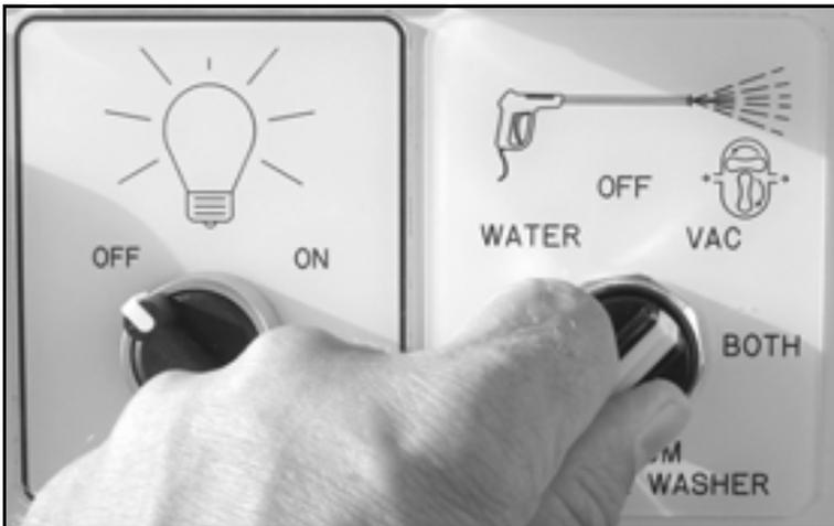
*Figure 5-13. Turn the Vacuum/Pressure Washer switch to the VAC position.*
