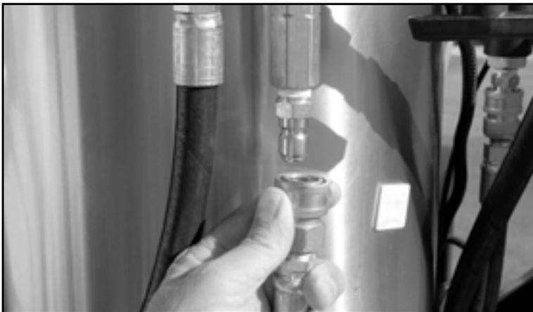
*Figure 4-8. Connect the sprayer hose to the input fitting on the water heater.*
