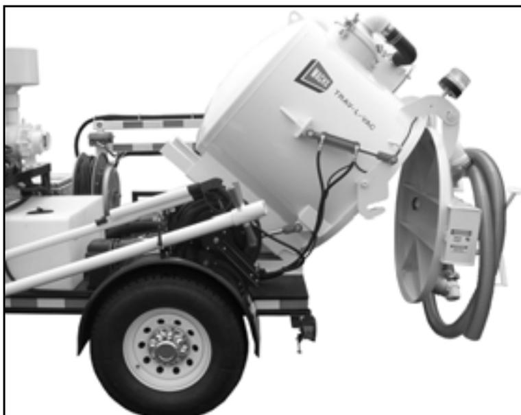
*Figure 5-26. Tank in the fully tipped position.*
