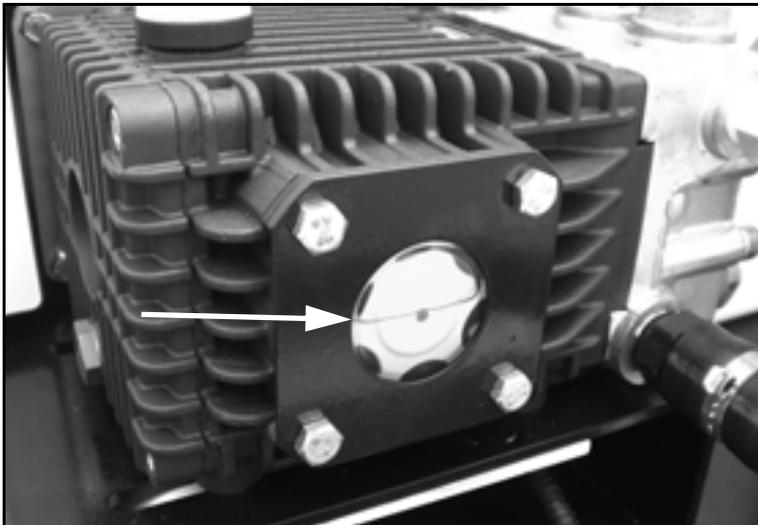
*Figure 6-13. Check the sprayer pump oil level using the sight glass on the side of the pump. The oil level should be at about the middle of the sight glass.*
