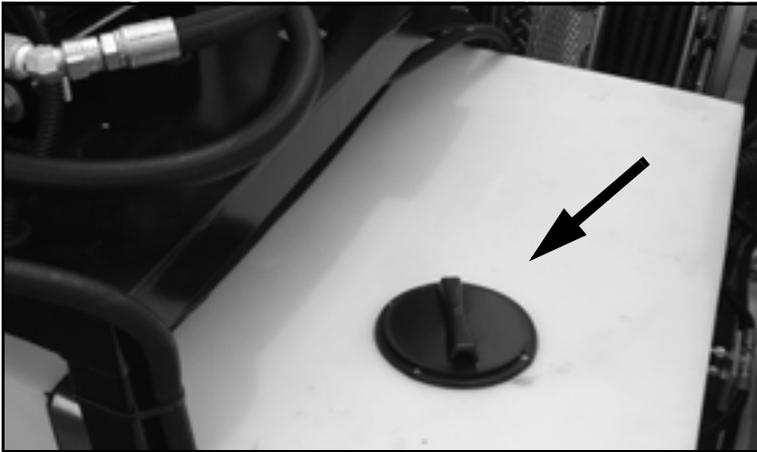
*Figure 5-31. The water tank cap; the water tank is at near the engine platform on the left side of the trailer.*
