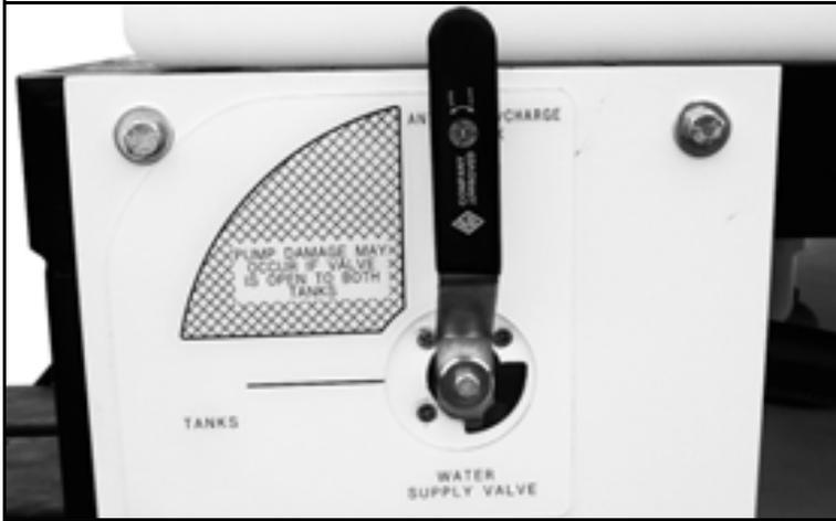
Figure 5-41. Move the Water Supply Valve to the ANTIFREEZE/CHARGE TANK position.
