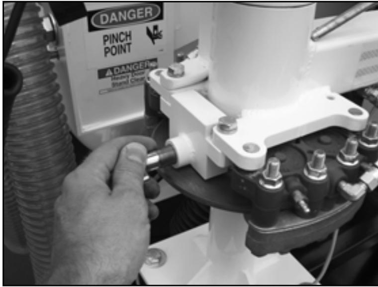
*Figure 5-63. Loosen the set bolt to move the arm.*
