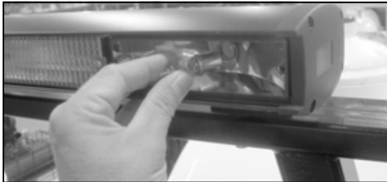
*Figure 7-34. Remove the light bulb from the socket.*
