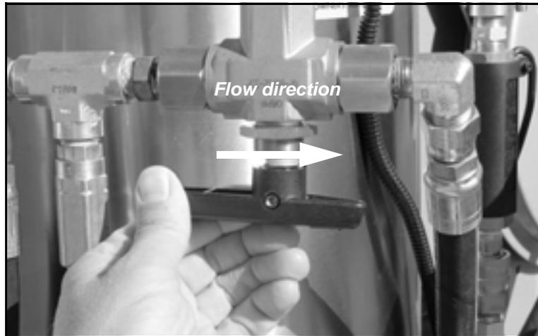
*Figure 5-55. The water flow through the water heater valve is toward the shorter end of the handle. To spray hot water, set the water flow to the right.*
