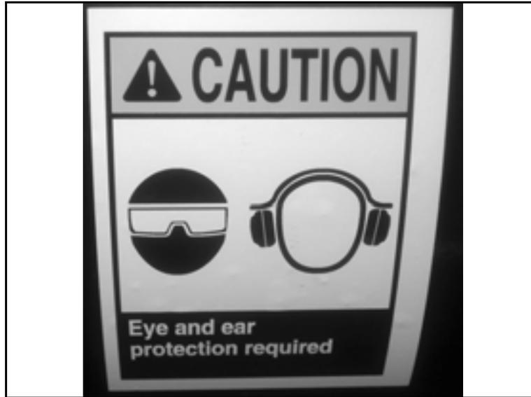
*Figure 2-1. The eye and ear protection label is on the vacuum filter cover, right-hand side of the blower belt guard, and on the door of the spoils tank (3 locations). Wear protective gear when operating the vacuum system. (Part no. 77-160-05.)*
