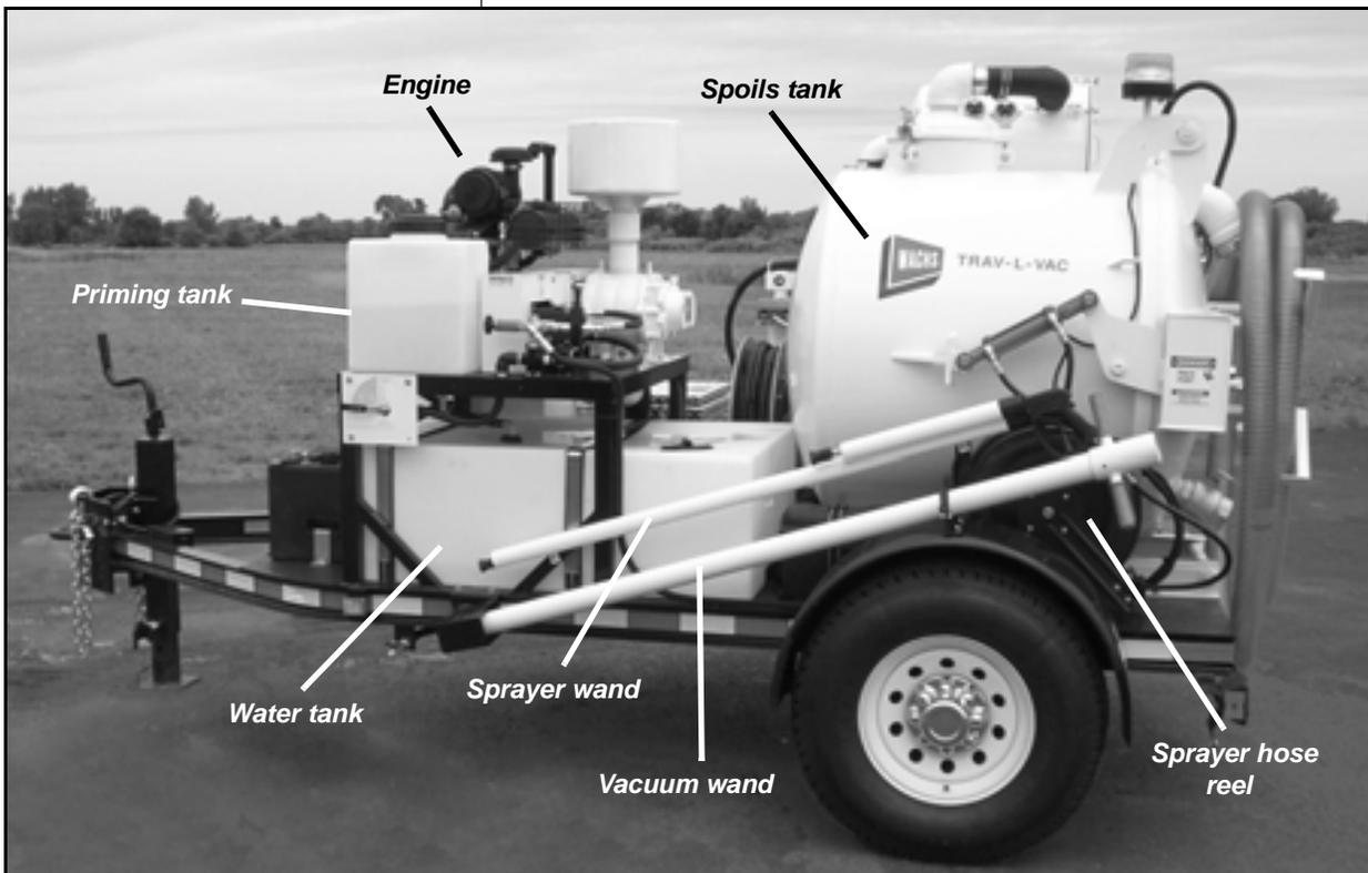
Figure 3-2. The left side of the VMT-2 trailer.
