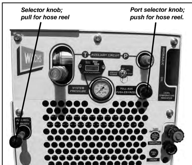
*Figure 5-47. To use the hydraulic hose reel, first push in the port selector knob labeled **PULL-AUX PUSH-ERV/REEL**, then pull the selector knob labeled **PULL-REEL PUSH-ERV**.*
