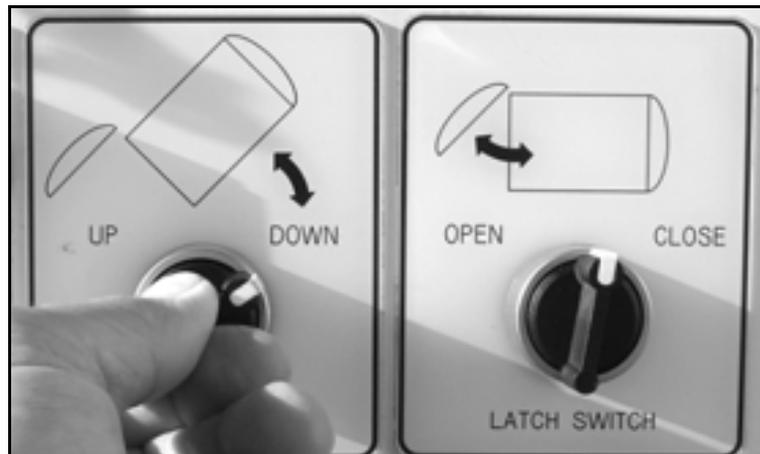
*Figure 5-21. Once the fluids have drained and the valves are closed, turn the Dump Switch to the DOWN position until the tank has moved back to its operating position.*
