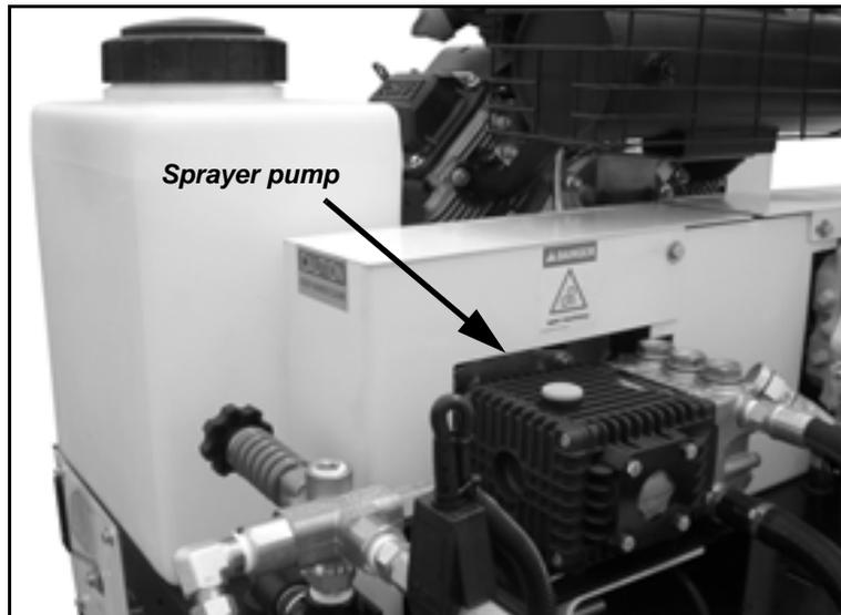
*Figure 3-11. The sprayer pump is opposite the cover behind the engine.*
