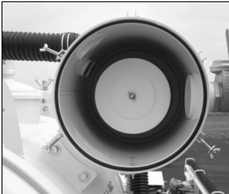
*Figure 3-8. The vacuum system filter canister shown with the clean-out door open.*
