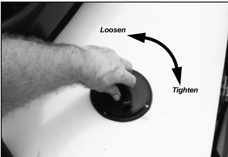
*Figure 5-32. Remove the cap to fill the water tank.*
