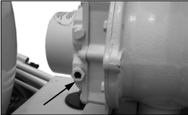
*Figure 6-12. Check the blower oil level using the sight glass on the side of the blower. Oil should be visible in the glass.*
