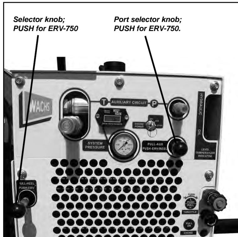
Figure 5-60. Push in both selector knobs to enable hydraulic flow to the ERV-750.
