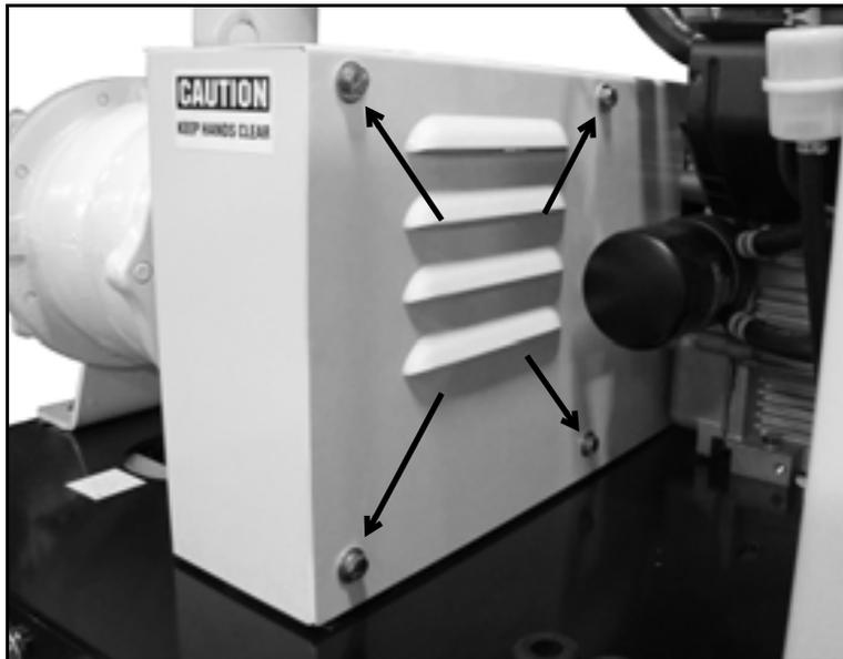
*Figure 7-16. Remove the four screws on the front of the blower belt cover.*
