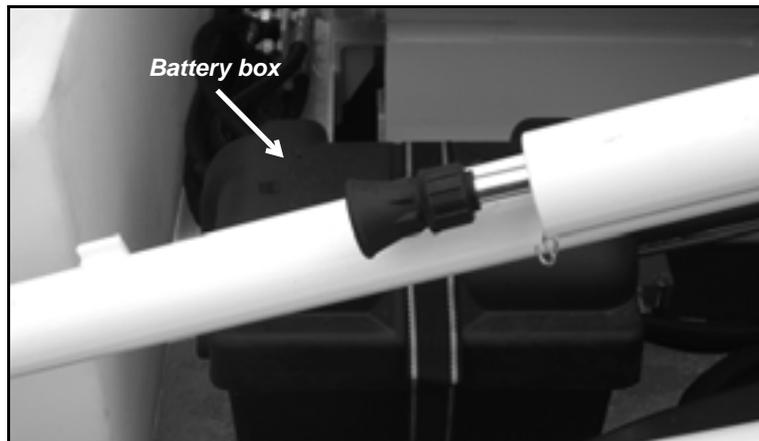
*Figure 7-31. Remove the strap and take the cover off the battery box.*
