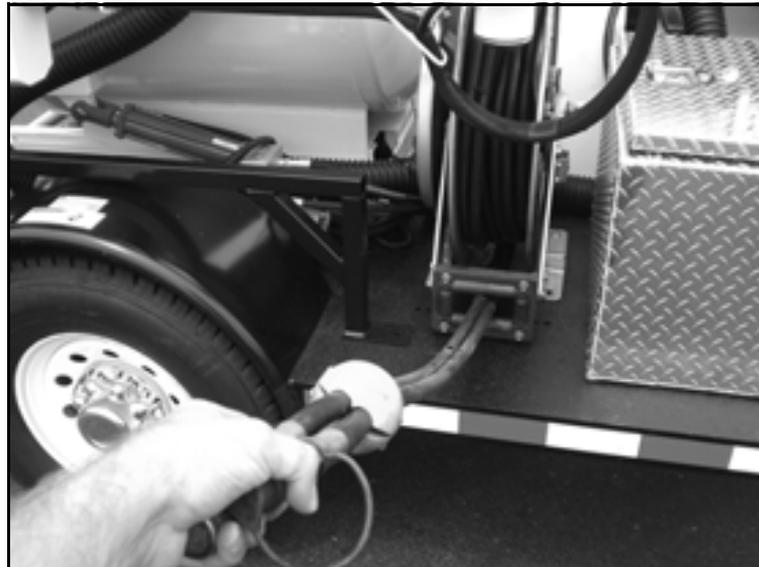
*Figure 5-49. Pull the hydraulic hose pair off the hose reel to the work location.*
