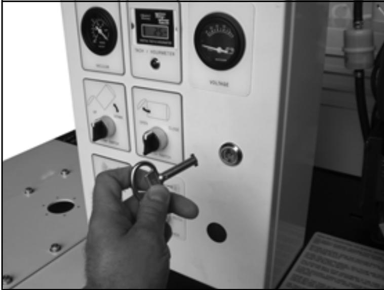
*Figure 7-14. Insert the key and turn to open the control panel cover.*
