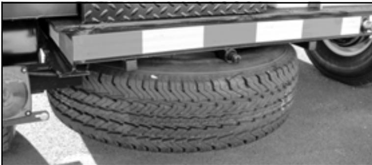
*Figure 3-16. The spare tire is mounted beneath the back of the trailer on a cable mechanism. To remove the tire, turn the cable drive nut with a 3/4" wrench or socket until the tire is on the ground.*
