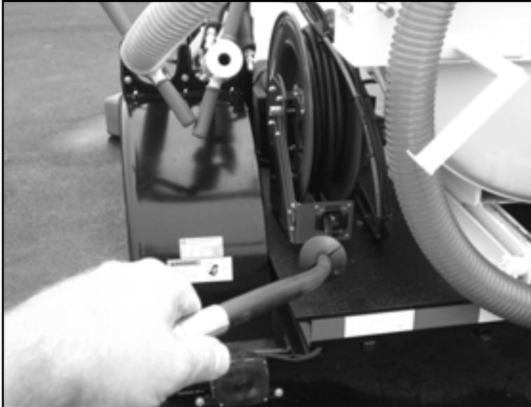
*Figure 5-34. Pull the sprayer hose out of the hose reel until it reaches the work location.*
