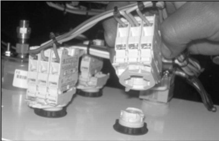
*Figure 7-12. Turn the locking ring to disassemble the switch for removal.*
