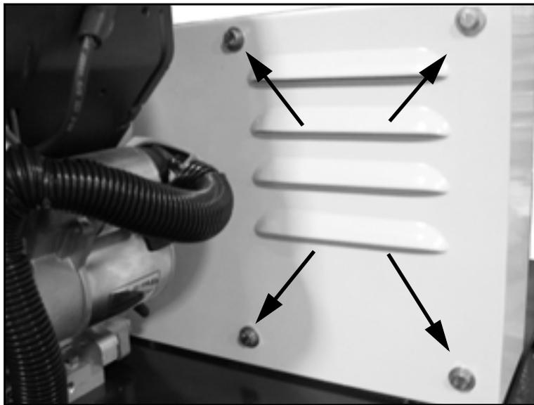
*Figure 7-22. Remove the four screws holding the front of the sprayer pump belt cover (shown with priming tank removed).*
