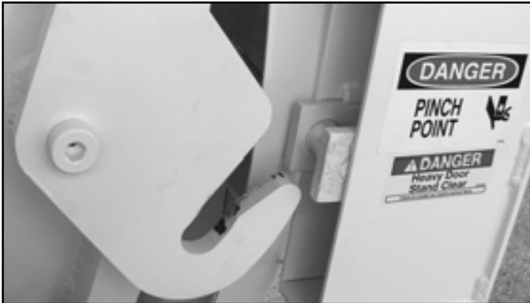
*Figure 7-25. When closing the tank door, the latch engages behind the latch pin to clamp the door shut.*
