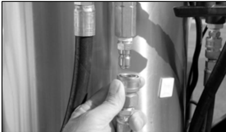
*Figure 5-58. Connect the hose from the reel to the inlet on front of the water heater.*
