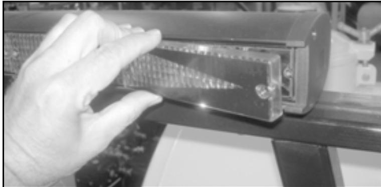
*Figure 7-33. Remove the two screws and pull the cover off the burned-out bulb.*
