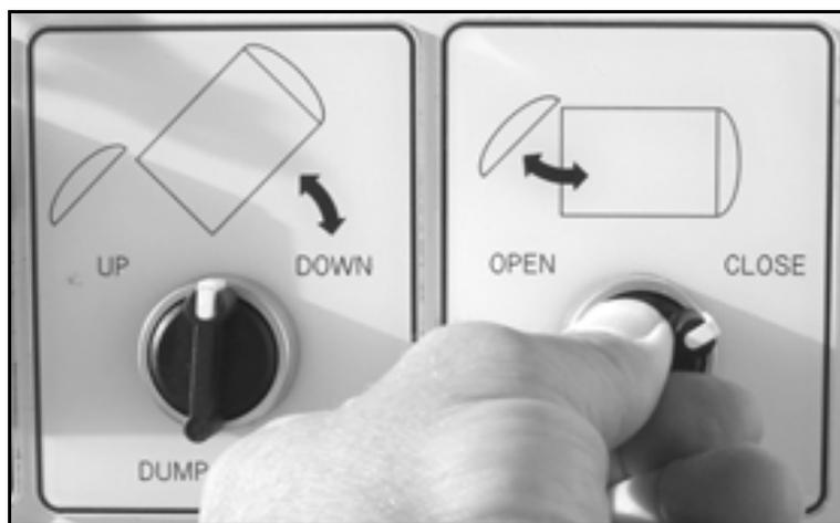
*Figure 5-28. When the tank is in the down position, turn the Latch Switch to the CLOSE position until the latches are fully engaged.*
