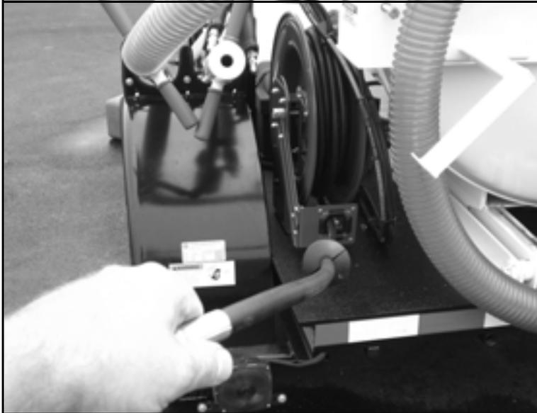
*Figure 4-7. Pull a sufficient length of hose from the sprayer reel to reach the front of the water heater.*
