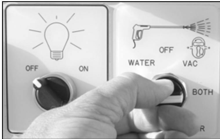
*Figure 5-14. To use both the washer and vacuum, turn the Vacuum/Pressure Washer switch to the BOTH position.*
