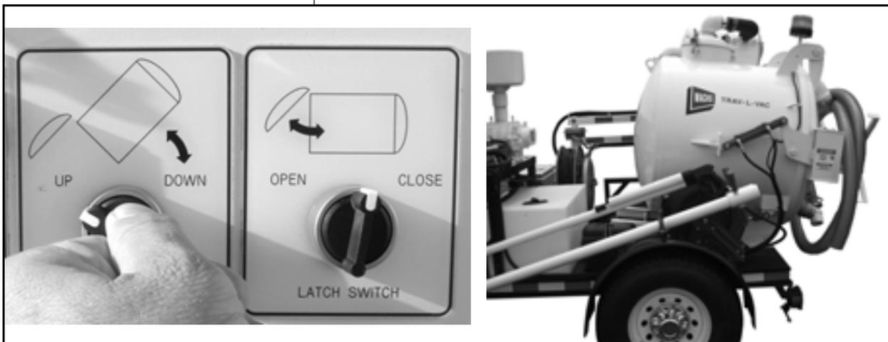
*Figure 5-17. Turn the Dump Switch to the UP position and hold it **just until the tank has cleared the deck and begins to tip**. Tip the tank approximately 10° - 20°.*
