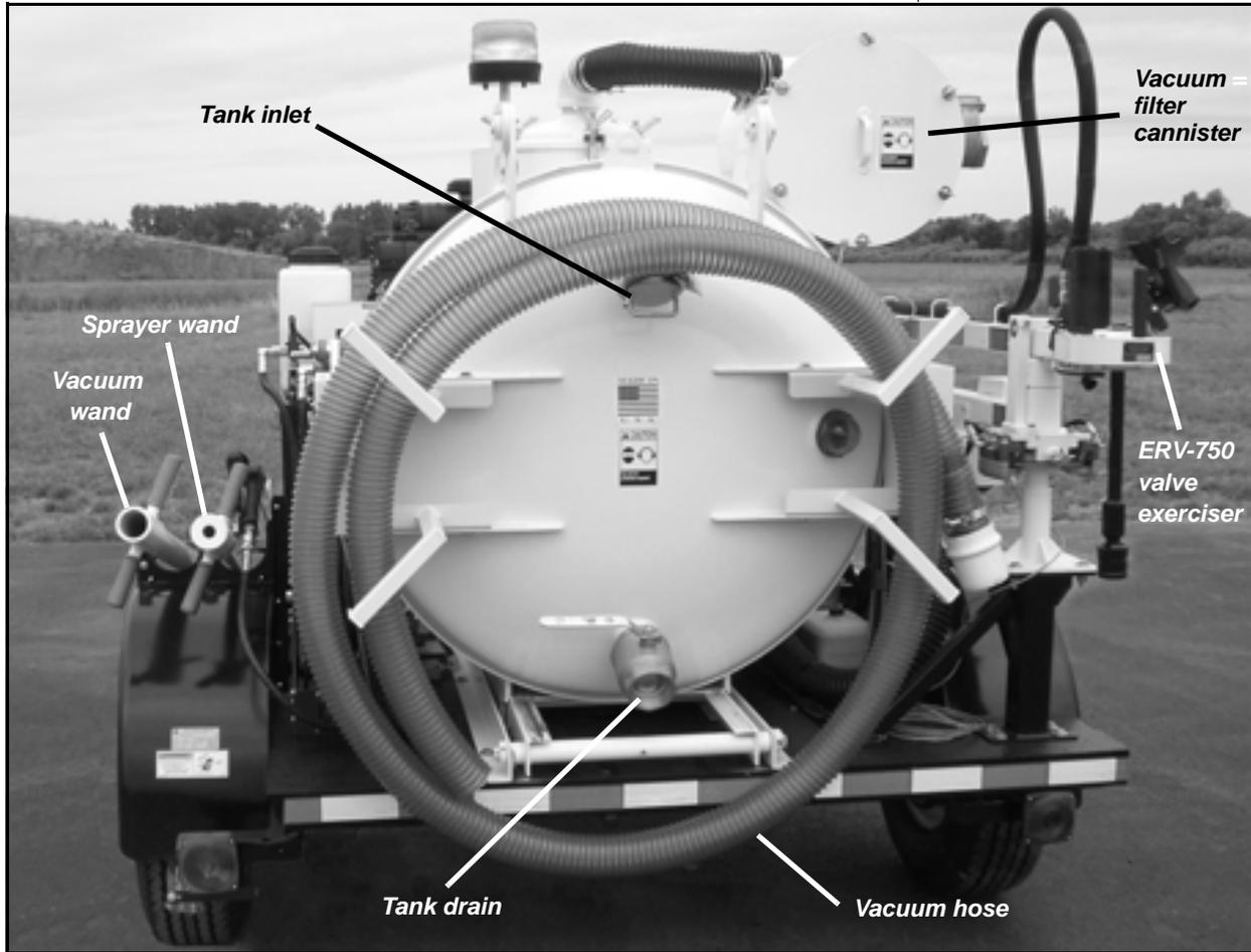
Figure 3-3. The back of the VMT-2 trailer.
