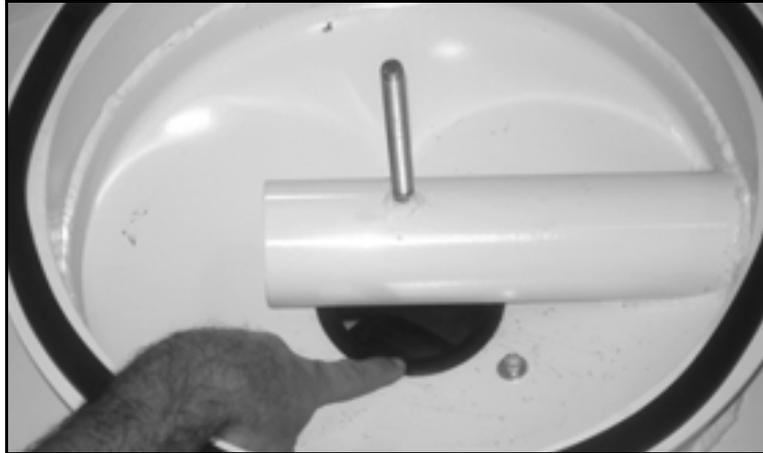
*Figure 7-5. The seal is in the vacuum port. Pry the old seal out and press the new seal in.*
