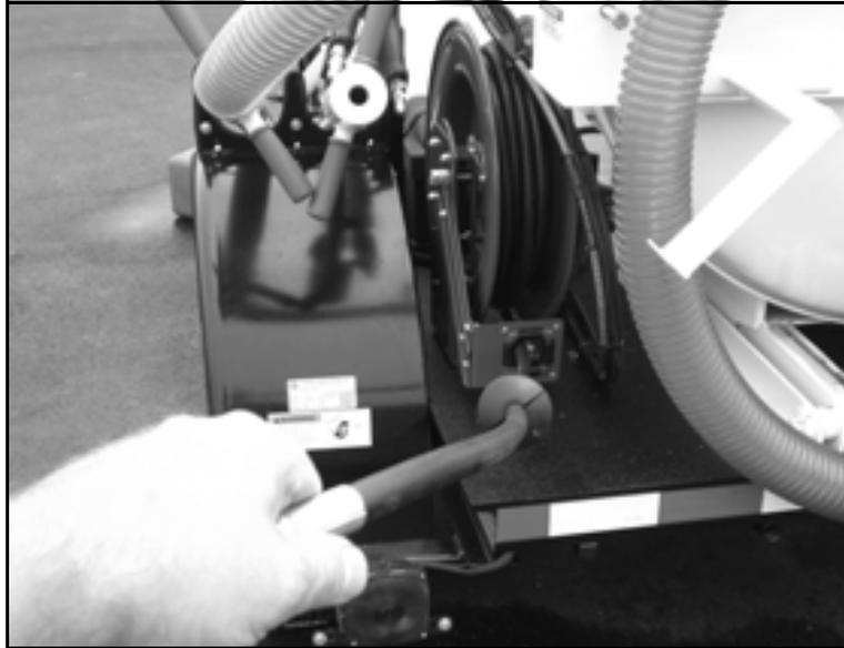
*Figure 5-57. Pull enough hose out of the sprayer reel to reach the front of the water heater.*
