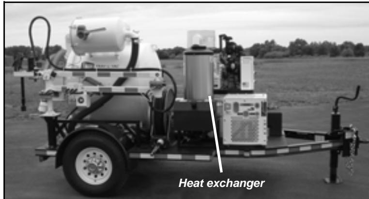
*Figure 3-17. The VMT-2 trailer with the optional water heater.*
