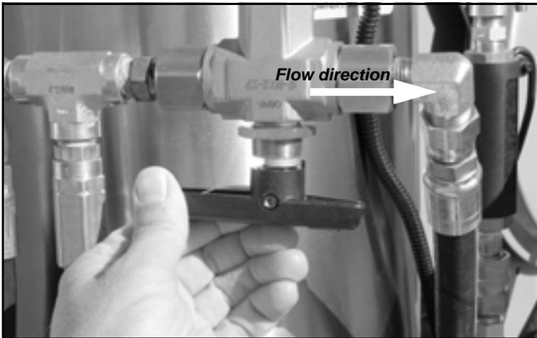
*Figure 5-59. Set the flow direction to the right to circulate hot water throughout the sprayer system.*
