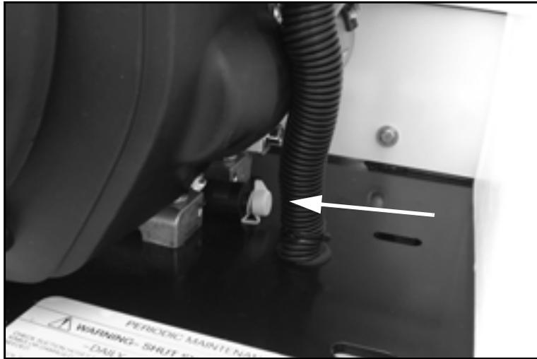
*Figure 6-18. Attach the hose to the drain valve on the gas engine. Press the valve in and turn to open it.*
