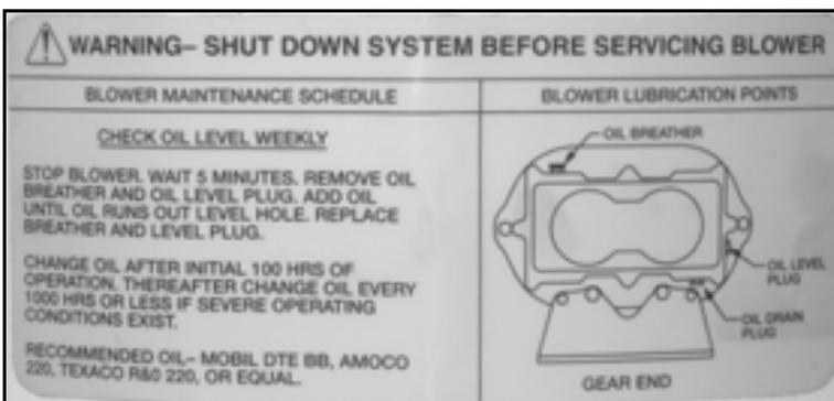
Figure 2-10. This warning label is on the blower silencer housing. Shut down the system when servicing the blower. (Part no. 67-111-00.)
