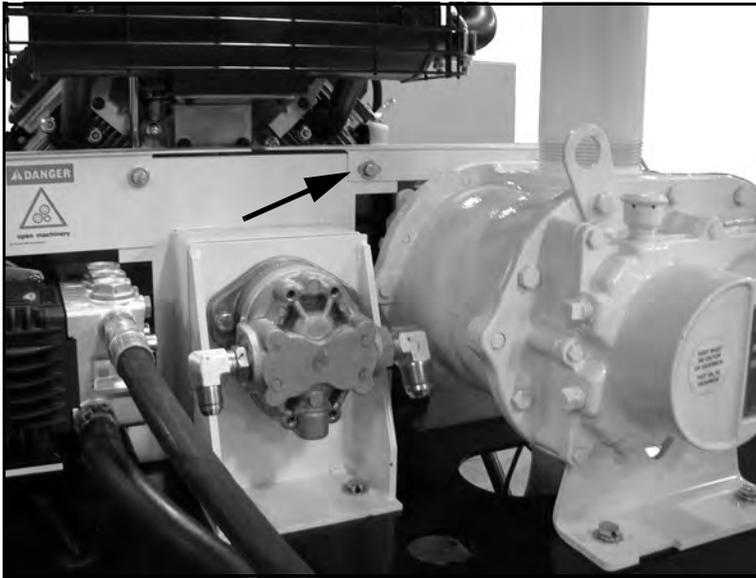
*Figure 7-17. Remove the one screw from the rear of the belt guard.*
