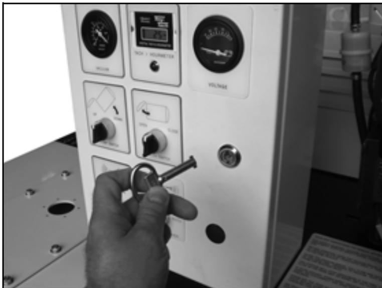
Figure 7-7. Insert the key and turn to open the control panel cover.
